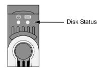
Figure 11. VTrak M500f/i/p disk carrier LEDs
